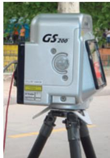
FIG. 6. Trimble GS200 TLS.
